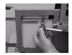
2. Cut the wire tie from the wire bundle in the rear of the unit, just above the condenser.
